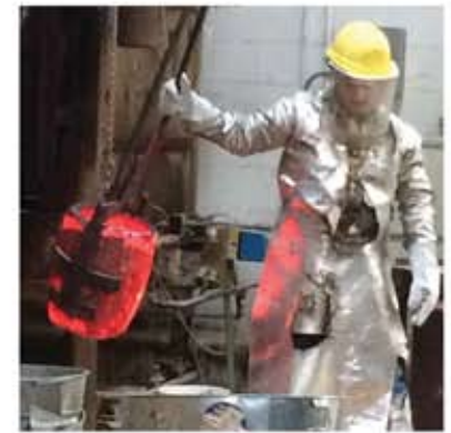
METAL POURED: Molten bronze is poured into the ceramic shell, and then is left to cool.
